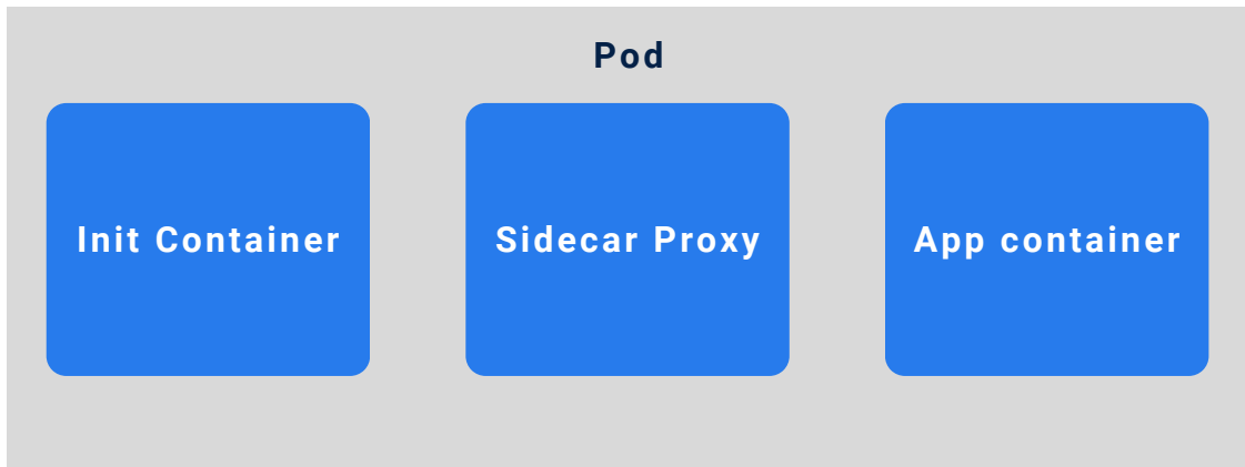
Fig E: The image highlights the containers inside a Kubernetes pod which is Istio-enabled.
